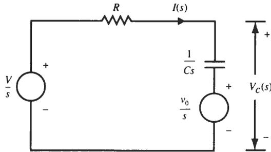
Fig. 3-15 Transform circuit.
