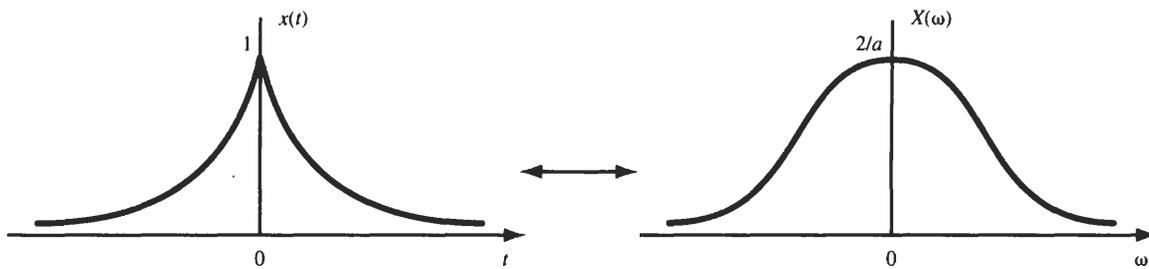
Fig. 5-18  $e^{-a|t|}$  and its Fourier transform.
