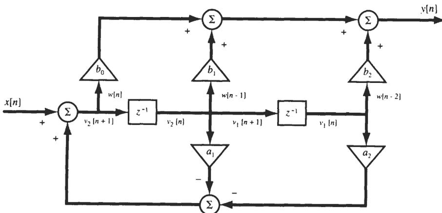
Fig. 7-9 Canonical simulation of the second form.
