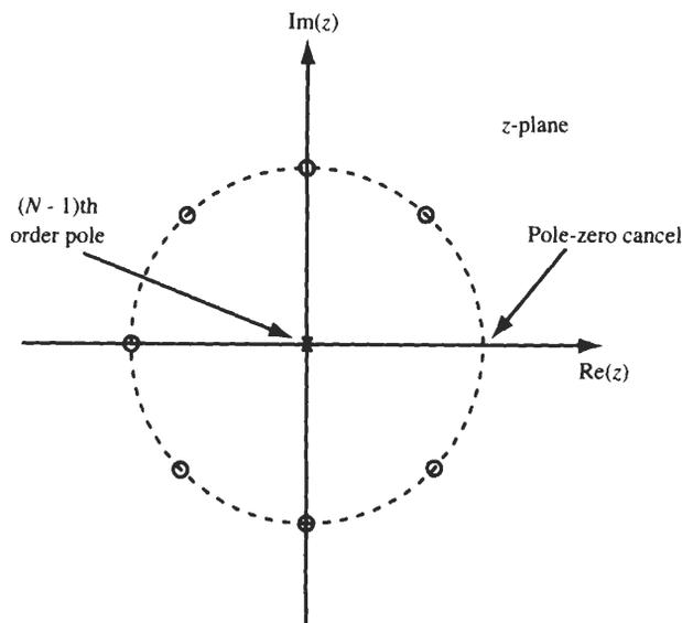
Fig. 4-4 Pole-zero plot with  $N=8$ .
