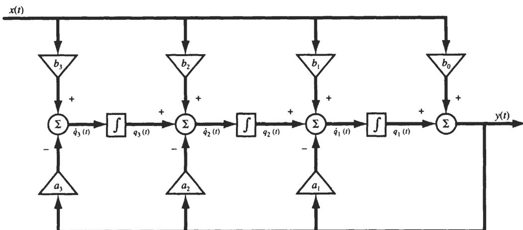
Fig. 7-14 Canonical simulation of the first form.
