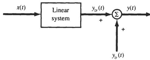
Fig. 2-2 Zero-state and zero-input responses.
