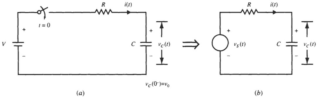
**Fig. 3-14**  $RC$  circuit.
