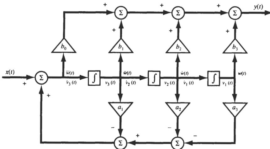
Fig. 7-16 Canonical simulation of the second form.
