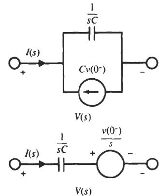
**Fig. 3-10** Representation of Laplace transform circuit-element models.
