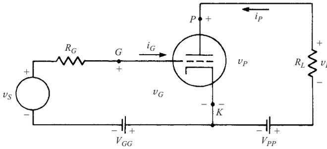
Fig. 4-14 Basic triode amplifier
