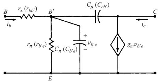
Fig. 8-8 Hybrid- $\pi$  model for the BJT
