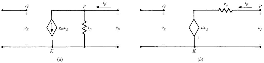
Fig. 7-9 Triode small-signal equivalent circuits
