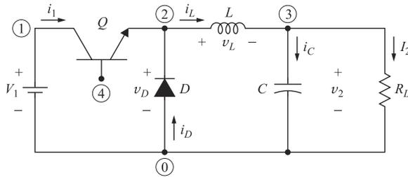
**Fig. 10-2** Buck converter
