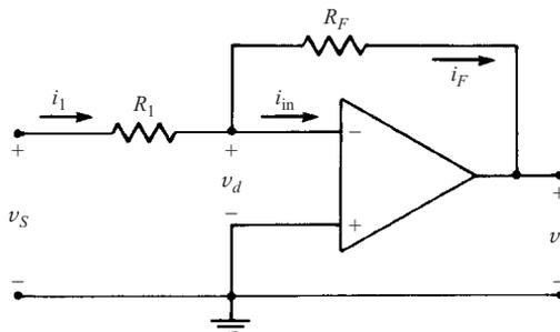
**Fig. 9-2** Inverting amplifier
