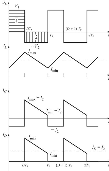
**Fig. 10-7** Buck-boost converter waveforms
