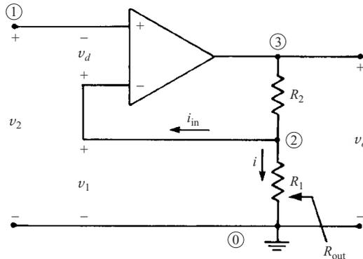
Fig. 9-3 Noninverting amplifier
