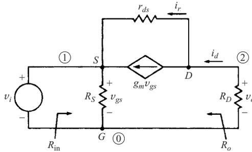
Fig. 7-4 CG small-signal equivalent circuit
