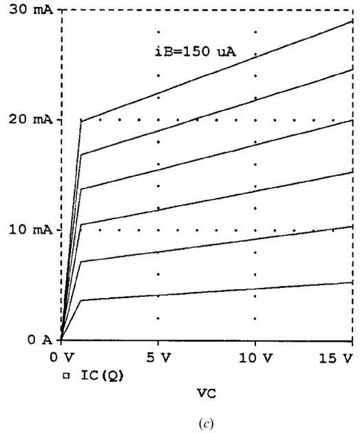
(b) Edit (Ex3\_2.CIR) to move the leading asterisks up one position on both the transistor specification statement and the .MODEL statements. Execute the revised (Ex3\_2.CIR) and use the Probe feature of PSpice to produce the collector characteristics for the generic BJT model (QNPNG or QPNPG) as displayed by Fig. 3-5(c).
