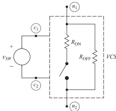
**Fig. 10-8** Voltage-controlled switch
