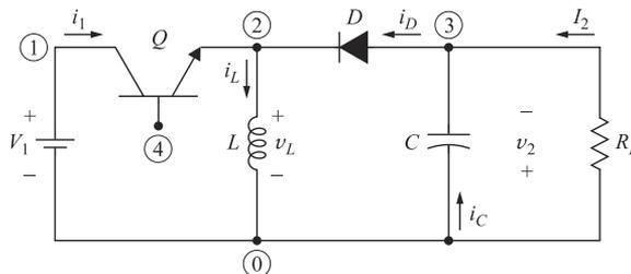
Fig. 10-6 Buck-boost converter
