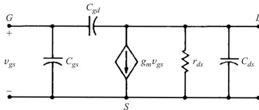
Fig. 8-10 High-frequency small-signal current-source FET model
