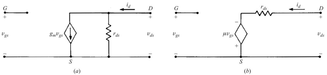
Fig. 7-1 Small-signal models for the CS FET
