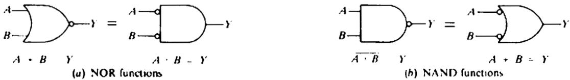
Fig. 5-14 Applications of De Morgan's theorems
