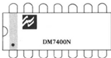
Fig. 6-36 Dual-in-line package IC
