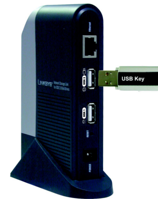
Figure 3-2: Flash Drive Connection
