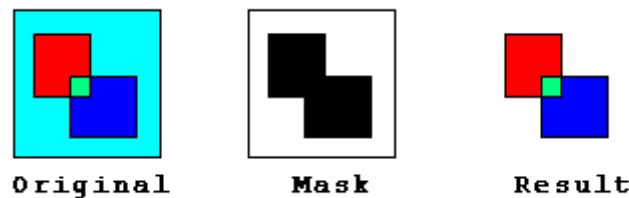
Figure 4.5 Example of using a mask to draw a transparent bitmap.
