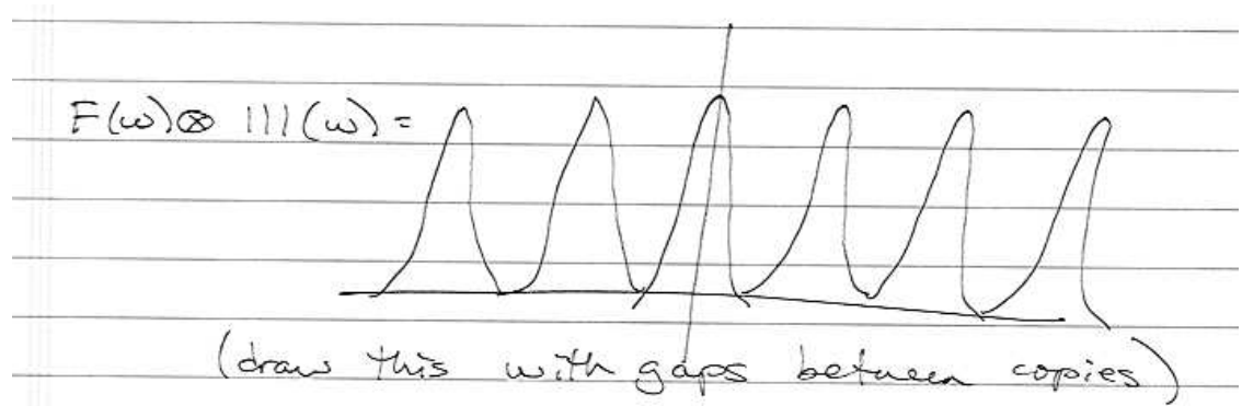
Figure 7.6: The convolution of F(\omega) and our shah function, resulting in infinitely many copies of the function F .
