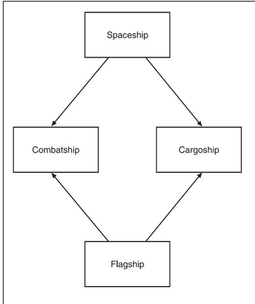
**Figure 5.2** *Diamond inheritance*, in which two classes share a common base class.
