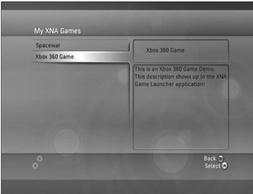
FIGURE 2.7 XNA Game Launcher reads the title and description values entered in the AssemblyInfo.cs file of the XNA applications we deploy.
